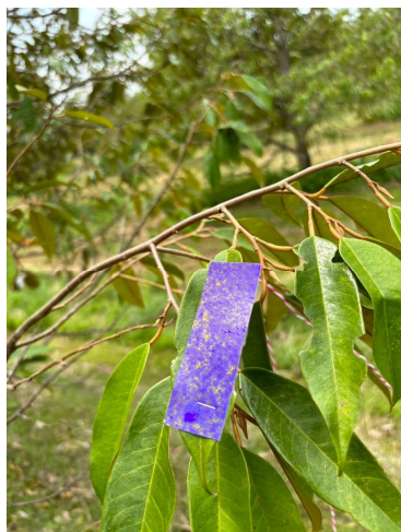
Figure 5: Water-sensitive paper was placed on a durian leaf to assess the coverage by an air blast sprayer.
