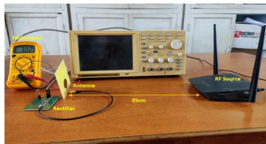
Figure 14: The established apparatus's calibration setup (Prashad et al., 2023)
