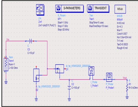
Figure 3: Simulated circuit to find Zin.
