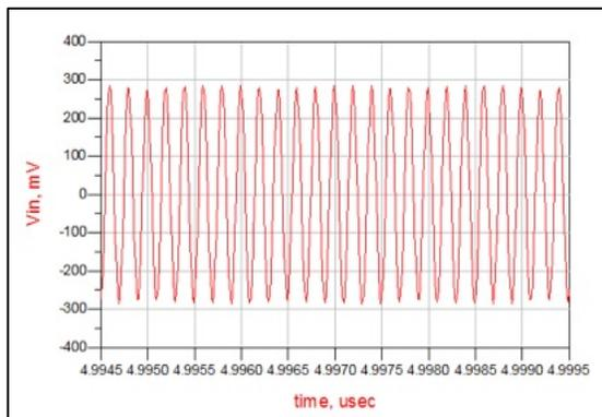
Figure 26: Vin (V) of rectifier circuit at 5 GHz with LC-Circuit.
