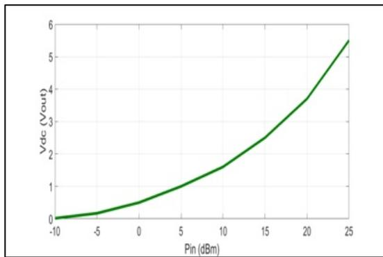
Figure 22:  $V_{out}$  (V) versus  $P_{in}$  (dBm) of Rectifier Circuit at 3.6 GHz with LC-Circuit.
