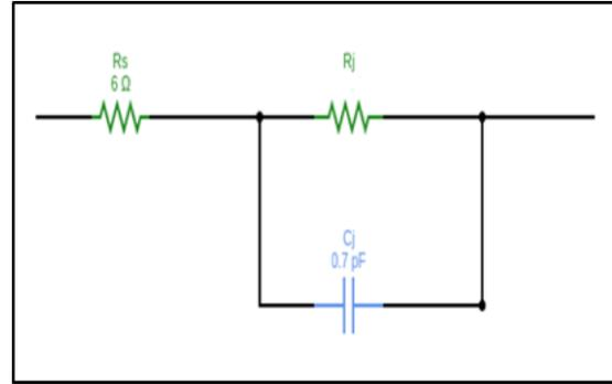
Figure 6: Equivalent Circuit for Diode.
