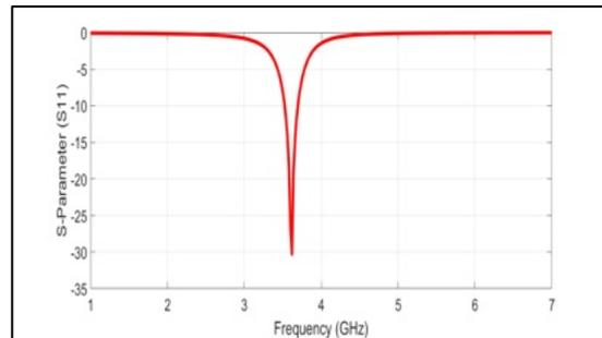
Figure 18: Simulated S11 of Rectifier Circuit at 3.6 GHz with LC-Circuit.
