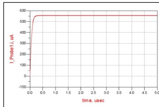
Figure 28: Output current of rectifier at 5 GHz with LC-Circuit.
