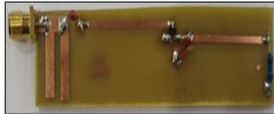
Figure 53: Photo of the front layer of the rectifier circuit.
