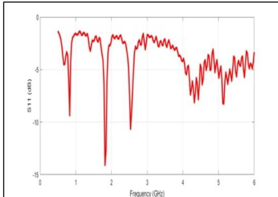
Figure 55: Measured S11 for the fabricated rectifier circuit.
