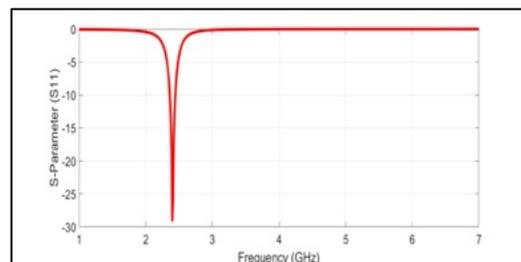
Figure 11: Simulated S11 of rectifier circuit at 2.4 GHz with LC-Circuit.
