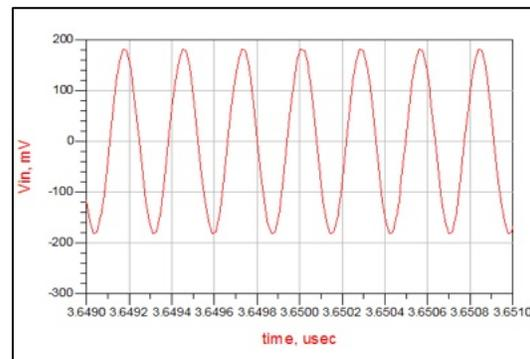
Figure 19: Vin (V) of Rectifier Circuit at 3.6 GHz with LC-Circuit.
