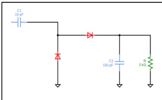
Figure 5: Rectifier Circuit.
