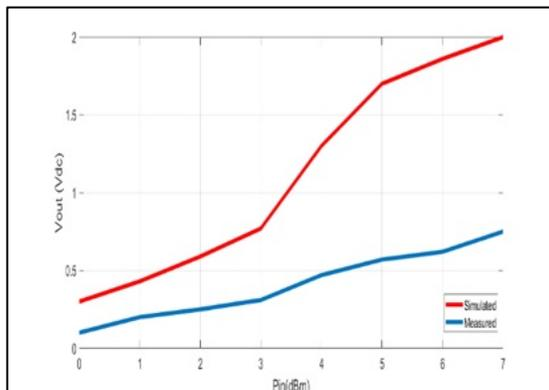
Figure 57: Comparison between simulated and Measured Vdc (Vout) versus Pin (dBm) at 3 kΩ.
