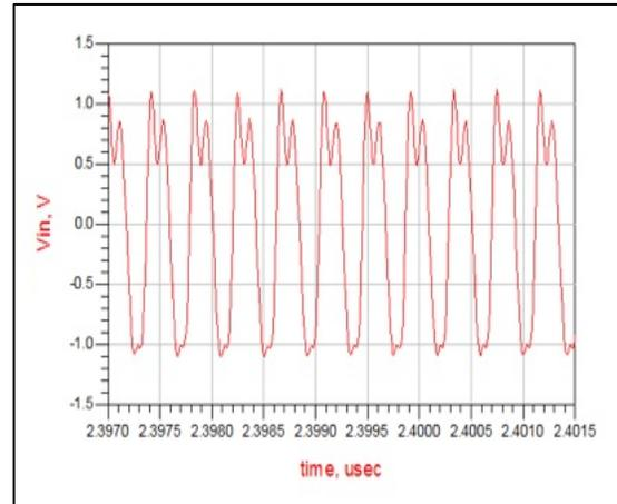
Figure 33: Vin (V) of Rectifier Circuit at 2.4 GHz with TL-Circuit.
