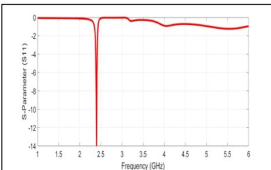
Figure 32: Simulated S11 of Rectifier Circuit at 2.4 GHz with TL-Circuit.
