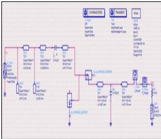
Figure 45: Rectifier circuit operating at 5 GHz with TL-Circuit.
