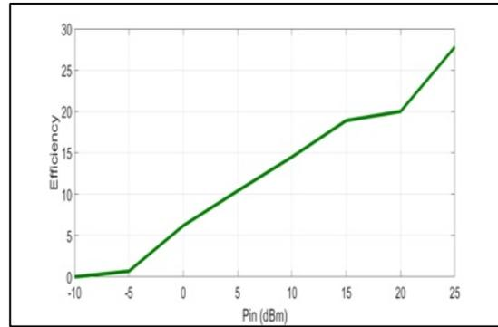
Figure 37: Efficiency versus input power of Rectifier Circuit at 2.4 GHz with TL-Circuit.
