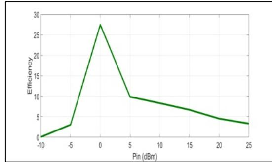
Figure 23: Efficiency versus input power of Rectifier Circuit at 3.6 GHz with LC-Circuit.
