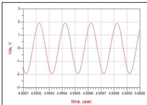
Figure 47: Vin (V) of Rectifier Circuit at 5 GHz with TL-Circuit.
