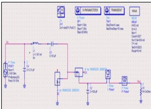
Figure 17: Rectifier circuit operating at 3.6 GHz with LC-Circuit.
