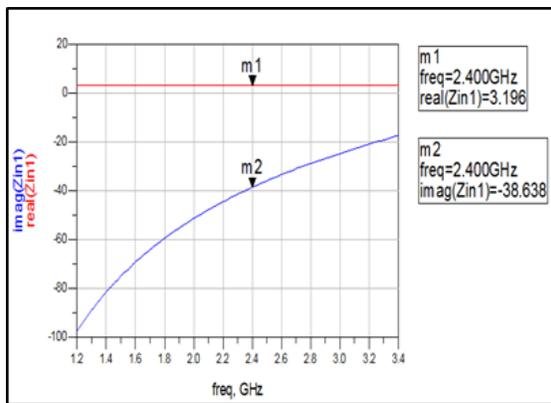
Figure 4: Simulated value of Zin
