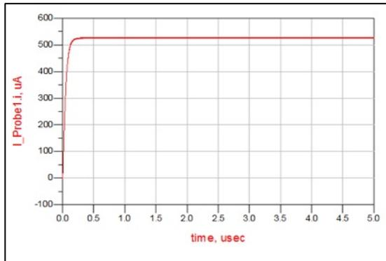
Figure 21: Output current of Rectifier Circuit at 3.6 GHz with LC-Circuit.
