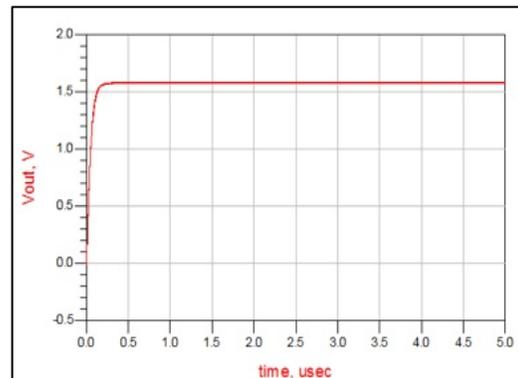
Figure 20: Vout (V) of Rectifier Circuit at 3.6 GHz with LC-Circuit.
