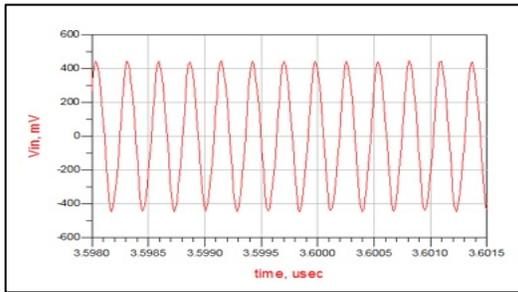
Figure 40: Vin (V) of Rectifier Circuit at 3.6 GHz with TL-Circuit.
