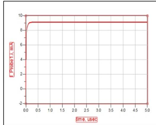
Figure 14: Output current of Rectifier Circuit at 2.4 GHz with LC-Circuit.
