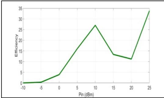
Figure 30: Efficiency versus input power of rectifier at 5 GHz.
