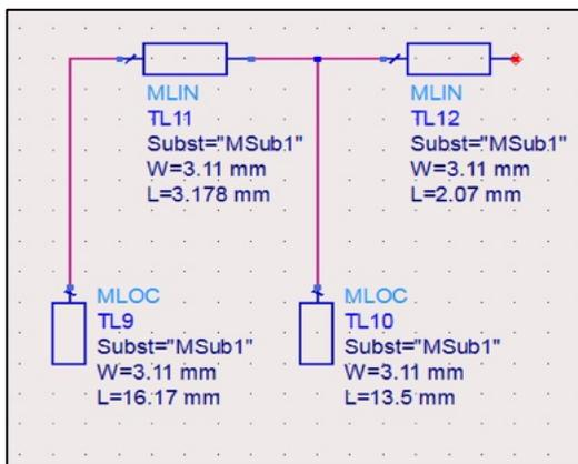
Figure 9: Simulated Block diagram of Transmission Lines (TL) at 2.4 GHz.
