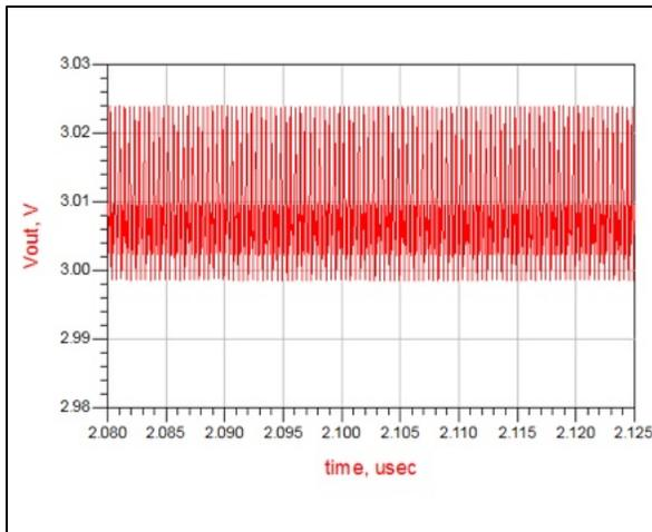
Figure 13:  $V_{out}$  (V) of Rectifier Circuit at 2.4 GHz with LC-Circuit.
