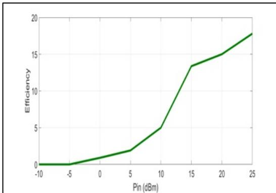
Figure 51: Efficiency versus input power of Rectifier Circuit at 5 GHz with TL-Circuit.
