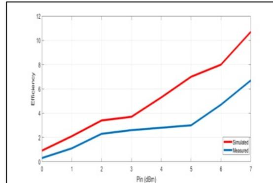
Figure 58: Comparison between simulated and Measured Efficiency ( $\eta$ ) versus Pin (dBm) at 3 kΩ.
