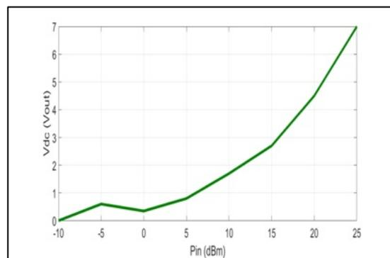
Figure 29: Vout (V) versus Pin (dBm) of rectifier circuit at 5 GHz with LC-Circuit.
