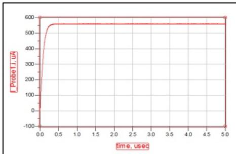
Figure 42: Output current of Rectifier Circuit at 3.6 GHz with TL-Circuit.
