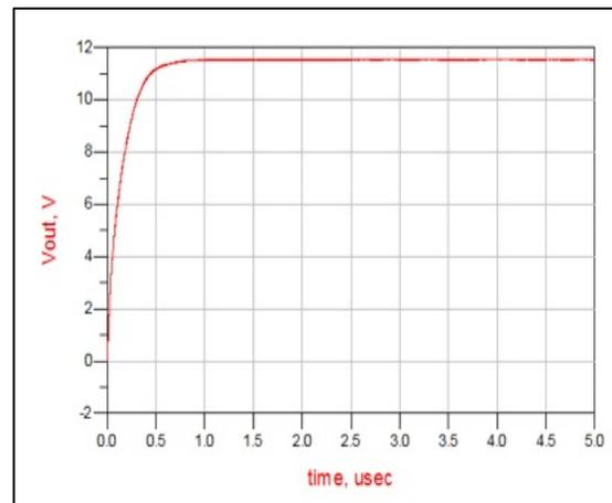
Figure 34: Vout (V) of Rectifier Circuit at 2.4 GHz with TL-Circuit.
