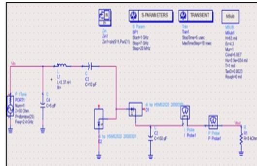
Figure 10: Rectifier circuit operating at 2.4 GHz with LC-Circuit.
