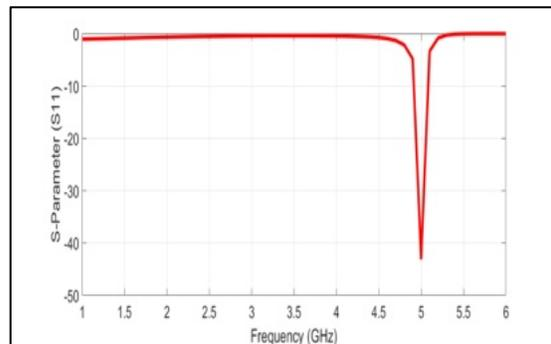
Figure 25: Simulated S11 of Rectifier Circuit at 5 GHz with LC-Circuit.
