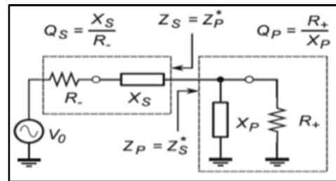
Figure 2: Equivalent Circuit for LC-Circuit.
