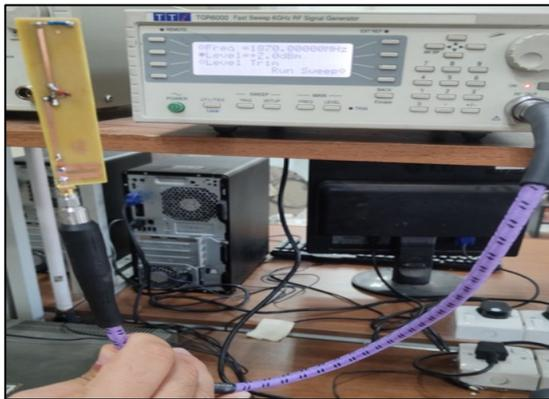
Figure 56: Photograph of the experimental setup showing the measurement of Vdc (Vout) Versus Pin (dBm).
