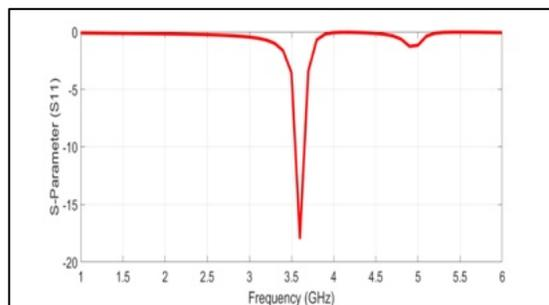
Figure 39: Simulated S11 of Rectifier Circuit at 3.6 GHz with TL-Circuit.
