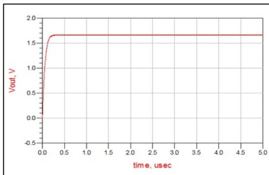
Figure 27: Vout (V) of rectifier circuit at 5 GHz with LC-Circuit.
