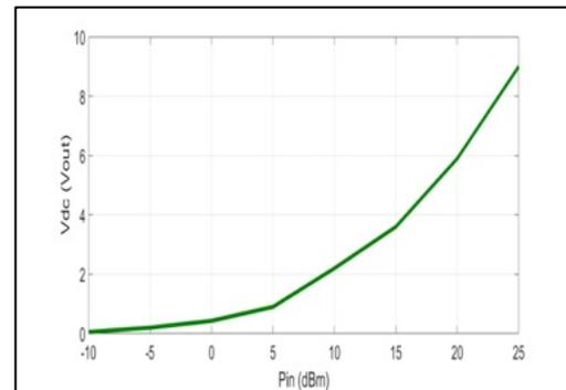
Figure 15:  $V_{out}$  (V) versus  $P_{in}$  (dBm) of Rectifier Circuit at 2.4 GHz with LC-Circuit.
