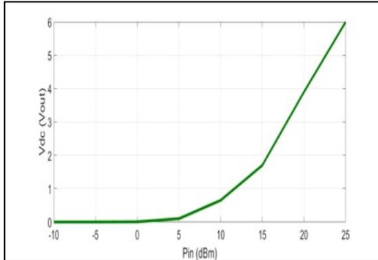
Figure 50: Vdc (Vout) versus input power of Rectifier Circuit at 5 GHz with TL-Circuit.
