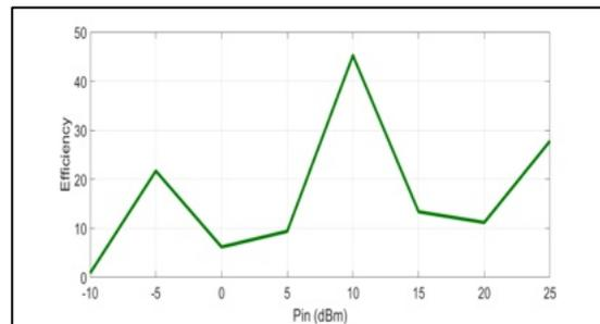
Figure 16: Efficiency versus input power of Rectifier Circuit at 2.4 GHz with LC-Circuit.
