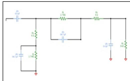
Figure 7: Analysis circuit to compute Zin.
