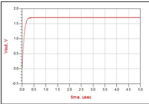
Figure 41: Vout (V) of Rectifier Circuit at 3.6 GHz with TL-Circuit.
