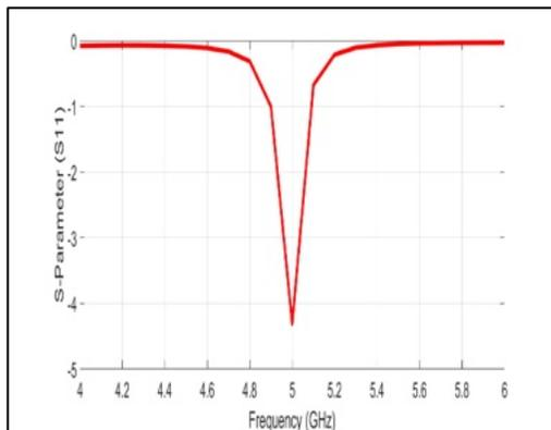
Figure 46: Simulated S11 of Rectifier Circuit at 5 GHz with TL-Circuit.
