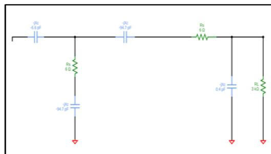
Figure 8: Final Analysis Circuit after neglecting  $R_j$
