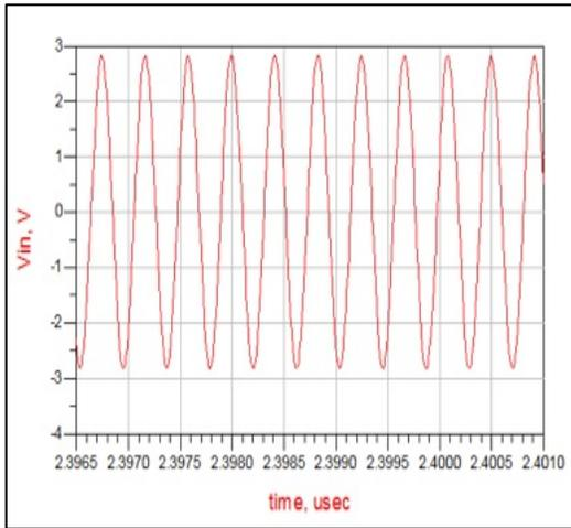
Figure 12:  $V_{in}$  (V) of Rectifier Circuit at 2.4 GHz with LC-Circuit.
