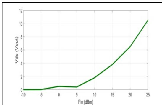
Figure 36: Vdc (Vout) versus input power of rectifier at 2.4 GHz with TL-Circuit.
