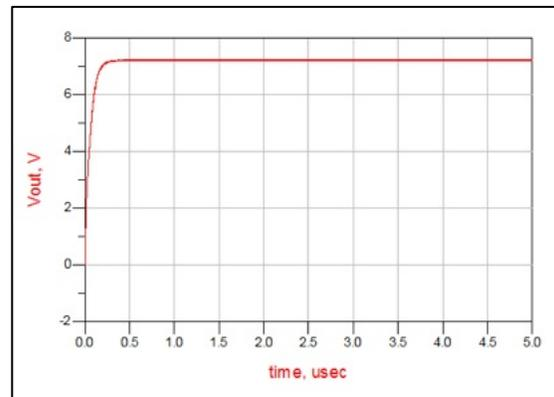
Figure 48: Vout (V) of Rectifier Circuit at 5 GHz with TL-Circuit.
