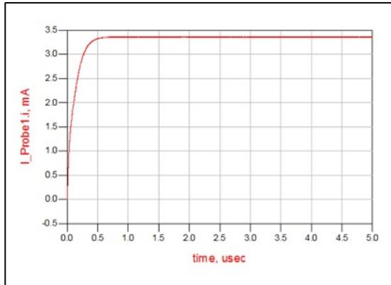
Figure 35: Output current of Rectifier Circuit at 2.4 GHz with TL-Circuit.
