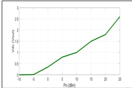
Figure 43: Vdc (Vout) versus input power of rectifier at 3.6 GHz with TL-Circuit.
