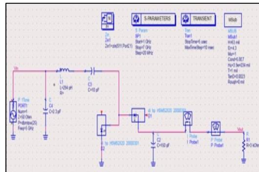
Figure 24: Rectifier circuit operating at 5 GHz with LC-Circuit.
