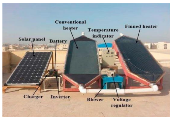
Figure 17: Solar air heater collector for different rib width and spacing with solar panel (Kabeel et al., 2018).
