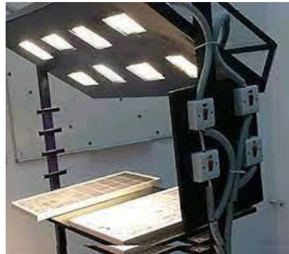
Figure 14: Solar simulator with halogen lamp (Moria et al., 2017).
