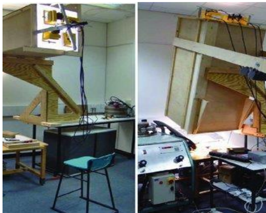
Figure 13: A halogen lamps solar simulator (Moss et al., 2017).
